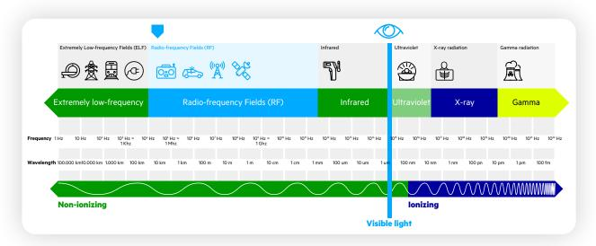
The image below shows the radio frequency fields including the different frequencies.
